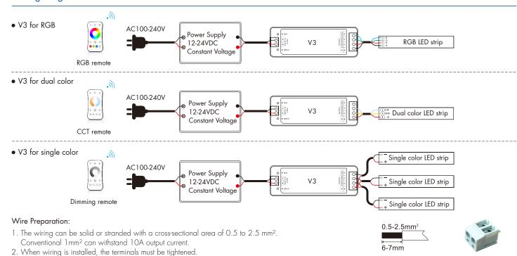
If they are not tightened, the contact point resistance will be too high and the terminals will easily burn due to heat when used at full load for a long time. Note: The output power of a constant voltage power supply should be at least 1.2 times that of the output load (light strip), otherwise the full power output of the load can easily cause automatic flickering or shaking of the light.
