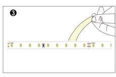
Tear off the double-sided adhesive tape on the back and paste it in a suitable position
