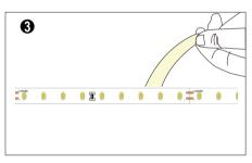
Tear off the double-sided adhesive tape on the back and paste it in a suitable position
