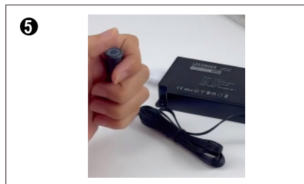
After the power supply and the switch are connected, the sensor switch can be used normally.
